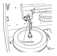
c. Lift the incubator cover to remove.
