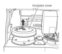
d. Unscrew the 5 screws on the upper incubator and remove the incubator.
