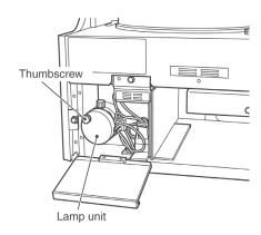
3. Unplug the connector of the light source lamp and remove the lamp unit.
