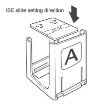
4. Set the slide cartridge with the label facing the outside of the sample carousel.
