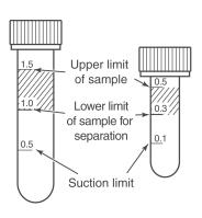
**NOTE:** The maximum number of tests that can be performed using a 0.3 ml whole blood sample in a 0.5 ml sample tube is five.
