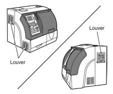
2. Remove all three louvers and pull out the air filter located inside of the louver. Lift the louver upward ▲ and then pull frontward ▼ to remove.
