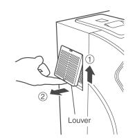
3. Remove dust adhering to the filter with a vacuum cleaner or running water.
