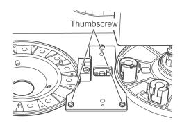
b. Unscrew the thumbscrew on the tip eject part and turn the tip eject part backward.
