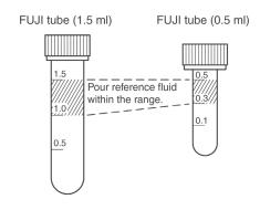
2. Replace reference fluid with a new tube containing new reference fluid.
