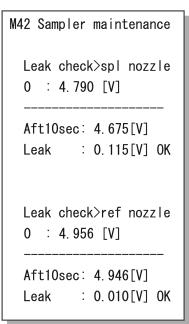
**NOTE:** Replace the sampler O-rings (Refer to *Section 5.6.*) when the test results are [NG].
