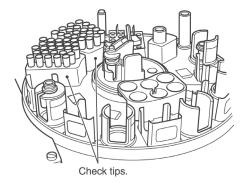
6. Remove the cap from the blood collection tube or sample tube which contains sample. Put the tube into the specified sample rack.
