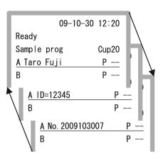
3. Press **PRINT**. The device will request detailed data on the current sample from PIMS and print the names of the requested tests.
