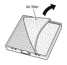
4. Insert the filter into the louver and put the louver back on the analyzer. Lift up the louver ▲ and then push it toward the analyzer ▼.
