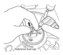
3. Wipe off the reference fluid cap using a cotton swab or soft gauze-like cloth moistened with distilled water. Dry it after cleaning.
