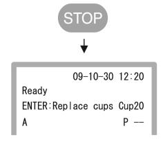
7. Press **TIP/CUP** to complete the replacement mode. The sample carousel turns the sample racks.
