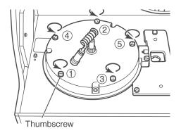
e. Wipe off the 13 pressure plates on the backside of the incubator with a soft gauze-like cloth or cotton swab moistened and tightly wrung out with sterilizing ethyl or isopropyl alcohol. Dry the pressure plates by facing the incubator backside (pressure plate surface) up.
