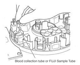
7. Check the sample type. Use SAMPLE to select P. The U, E and W indicators are not usable with Heska's current slide selection.
