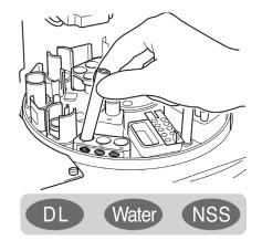
2. Make sure that [Warming up], [Ready] or [Spot interrupted] is displayed on the LCD (the analyzer is not in the process of sampling).
