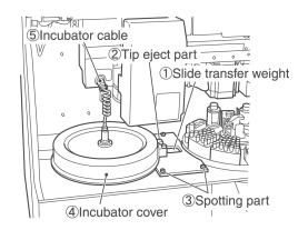
**NOTE:** To avoid stressing the cable, ensure that the incubator cable is not twisted. Otherwise, the cable will be damaged in a short time.
