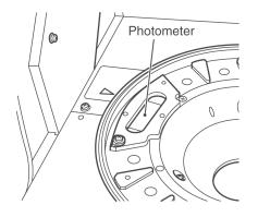
j. Remount the reference plate. Align the arrow mark on the reference plate with the arrow mark on the analyzer. Screw the 2 thumbscrews evenly.
