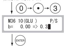
d. After completing the inputs of (a, b), the old values, the input values, and the new values are printed out.
