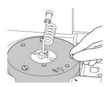
14. Reset incubator cover A and plug in the incubator cable. Pass the cable of incubator B through the hole in the center of incubator cover A. Align ▼ on the incubator cover with the ▲ mark on the analyzer.
