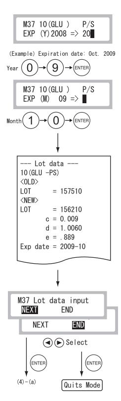
To reset coefficients for each test:
