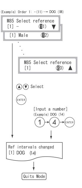
6.2.29 Mode 86 Editing and Inputting Reference Interval Names < Admin.> This mode is used to edit or input reference interval names.
