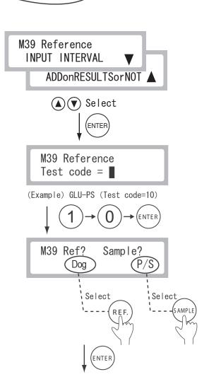
c. Input a lower limit value.After the input, press ENTER.
