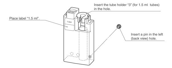
Using samples with sample tubes
