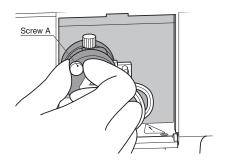
3. Unplug the connector of the light source lamp to remove the lamp unit.
