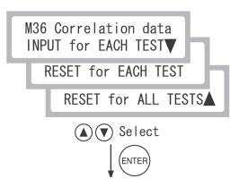
4. To input coefficients for each test:
