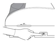
Remove the disposal box and dispose of the tips and slides.
